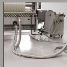
Electrical Heated Hose Pipe
