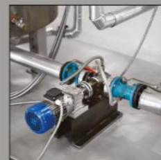
Gear Pump & Jacketed Valves
